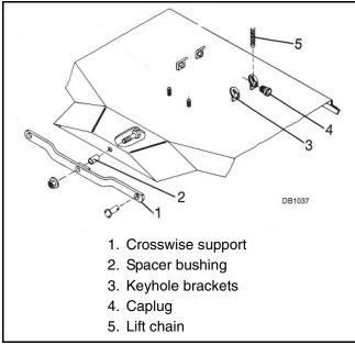
Figure 16. Crosswise Support Installation
